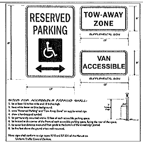
2 TYPICAL ACCESSIBLE PARKING SIGNAGE N.T.S.
